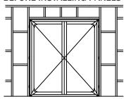
Measure the diagonals of the opening for the French door with a measuring tape. It is important for the correct operation of this product that the difference does not exceed 4mm.
