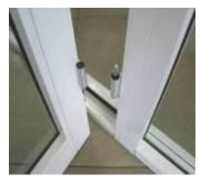
Sit the panel perpendicular to the door frame. This will ensure that the panel does not strike the head of the door frame when the panel is lifted up. The hinge knuckles should be facing each other (as indicated in the picture).
