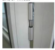
Locate the panel so that the panel hinge knuckles are positioned directly above the frame hinge knuckle pins. Make sure that all the hinges are lined up correctly.
