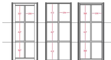
Illustration of a 1372mm high awning window. Windows 1800mm high or above come with 3 horizontal bars as standard.
