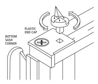
Sash slides on our windows and doors are height adjustable. To adjust the height on one or both of the slides, remove them and rotate higher or lower.
