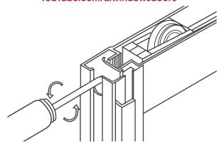
Slide the door to its almost closed position. Check that the door is plumb to its frame and clear of the track. If necessary one or both rollers may be adjusted by turning one or both of the adjustment screws clockwise to raise the door, and anticlockwise to lower. This adjustment can only be performed with all the weight of the door taken off the roller by holding the door panel jamb clear of the track.
